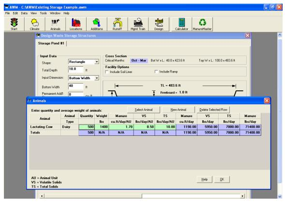
2. Now manipulate the number of animals in the animal screen to obtain the existing storage dimensions. As you change the animal numbers the storage dimensions will change in the design screen. For this example the storage pond is 10 ft deep, 3:1 sideslopes, 100ft x 200ft top dimensions. Through trial and error by changing the animal numbers you can get within .3ft of a foot to the actual storage dimensions of the existing structure.
