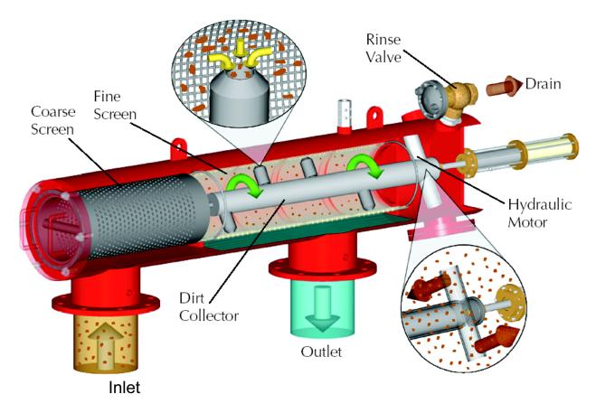
Figure 3. Automatic self-cleaning screen filter.
