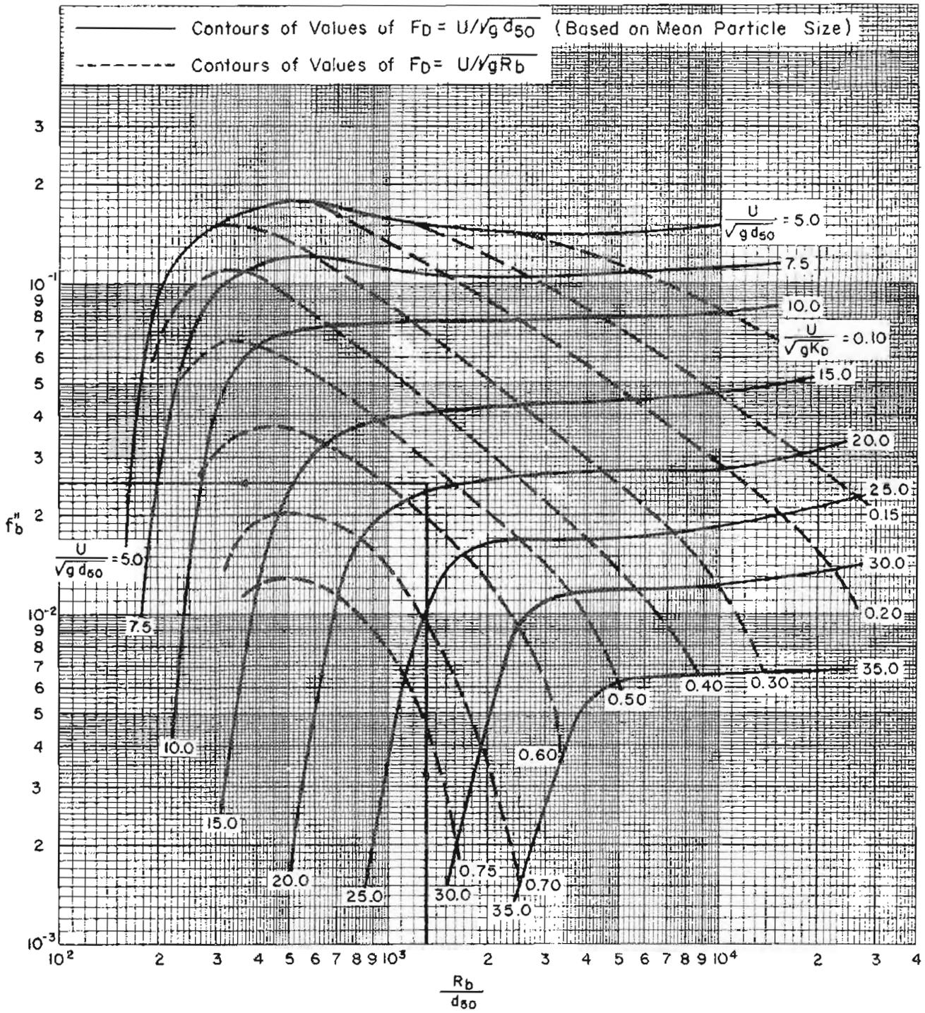
Figure 4-15.—Form-drag friction factor in sand-bed channels,  $f_b''$ , as a function of  $R_b/d_{50}$  and  $F_D = U/\sqrt{gd_{50}}$ . From Alam and Kennedy (1969), American Society of Civil Engineers (1975, p. 142).
