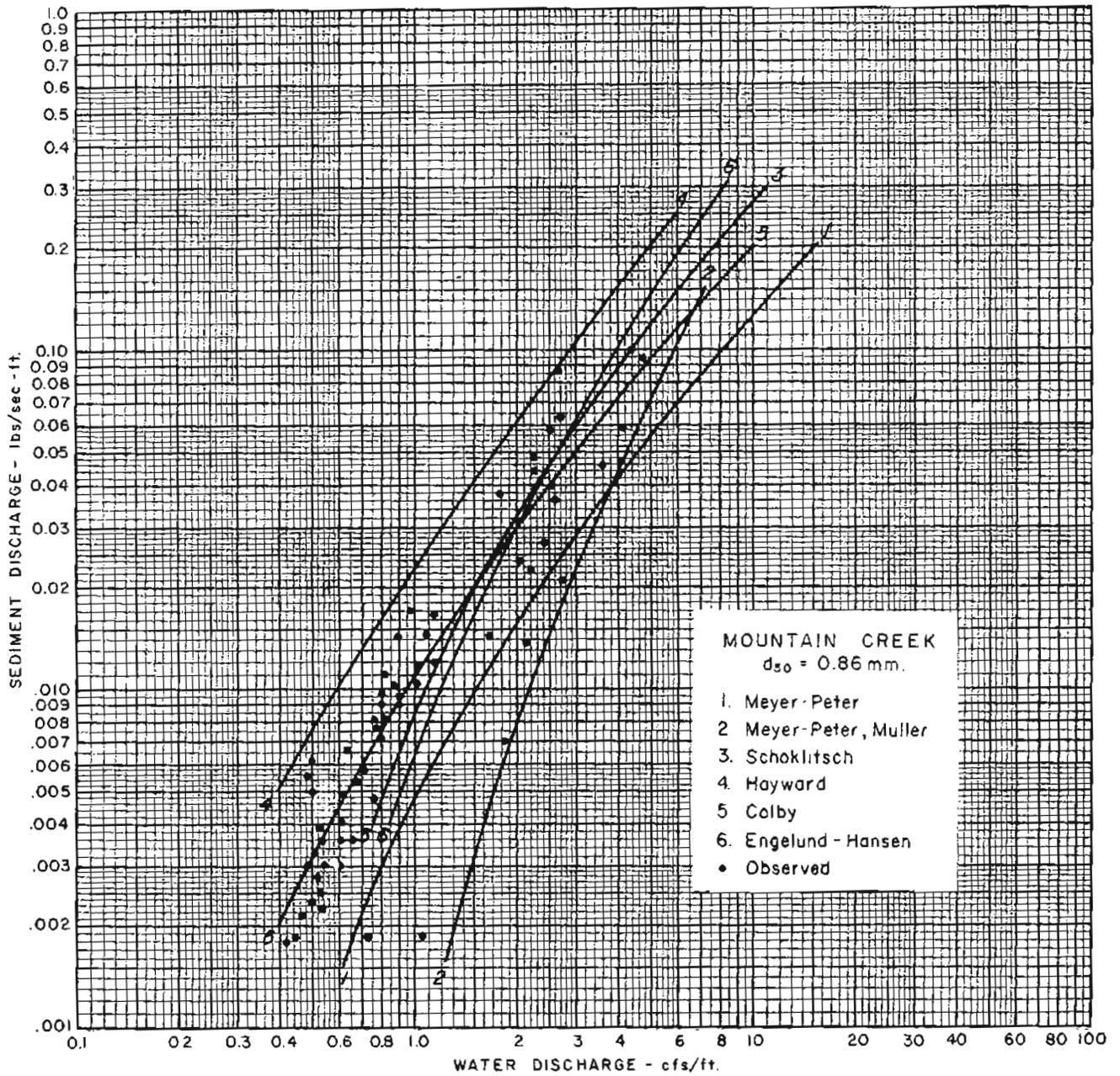
Figure 4-9.—Sediment rating curves for Mountain Creek near Greenville, S.C., according to several formulas compared with measurements. Adapted from Vanoni, Brooks, and Kennedy (1961, p. 7-8).
