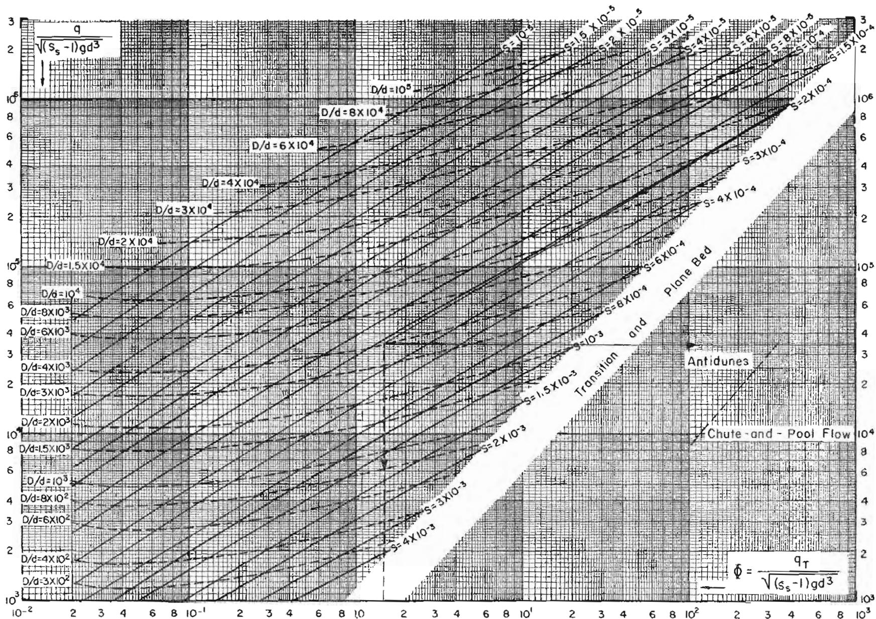
Figure 4-5.—Graphical solution to  $\sqrt{(S_s - 1)gd^3}$  and  $\phi$  in the Engelund-Hansen procedure. Adapted from Engelund and Hansen (1967) and American Society of Civil Engineers (1975, p. 209).
