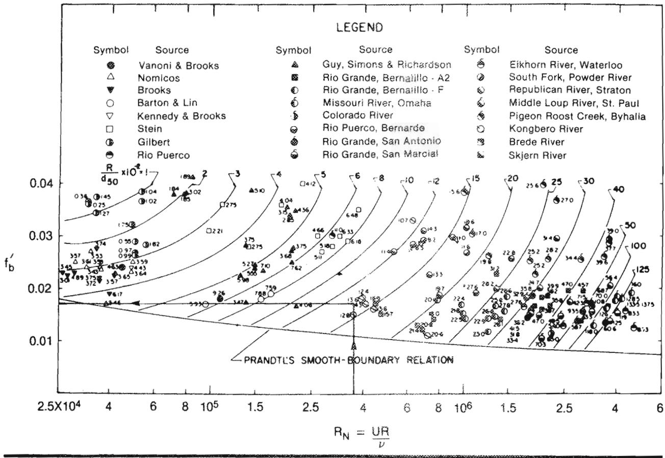
Figure 4-16.—Friction-factor predictor for flat-bed flows in alluvial channels. The number by each point is  $R/d_{50} \times 10^{-2}$ . From Lovera and Kennedy (1969), American Society of Civil Engineers (1975, p. 140).
